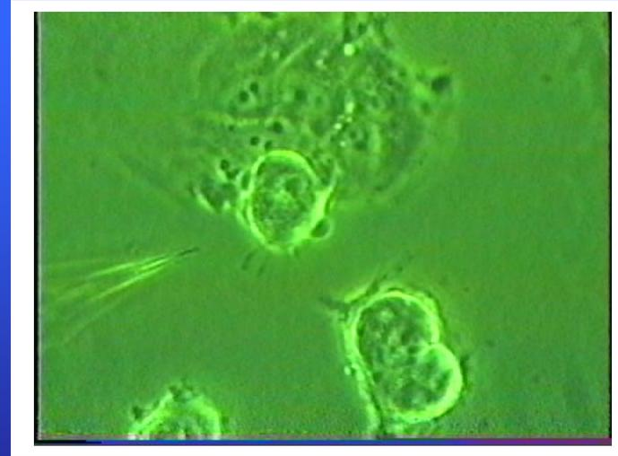
**LEFT TO RIGHT, single cell analysis, optical nanosensor outside MCF-7 cell (i) right before insertion into MCF-7 cell (ii) inserted into MCF-7 cell and (iii) extracted from MCF-7 cell**
