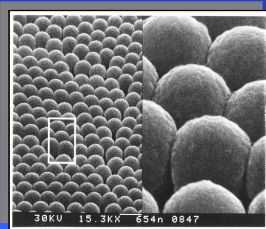
**SEM micrograph of silver-coated polystyrene microspheres**
