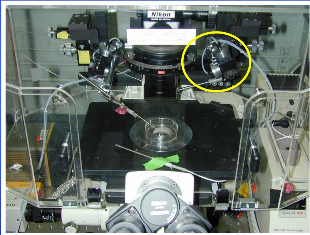
NIKON inverted fluorescence microscope
