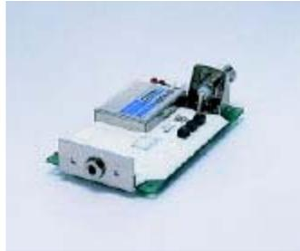
Figure 3.12 Hamamatsu APD module used for cw fluorescence detection *in vivo*.
